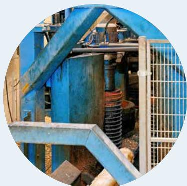
With advanced laser measurement and optimised algorithms, we measure the shape of the log with high precision and calculate the most efficient way to saw it. A number of different control systems capture results and ensure that no mistakes are made in the process. RemaSawco's smart control system provides an efficient flow with minimal downtime.
