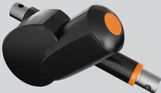
RE25 Compact, strong and robust. 360° stepless rotational motor and brackets for high flexibility in assembling and development. Max. push force: 5000N Build-in length: 110 mm + stroke IP-class: IPX 1-4
