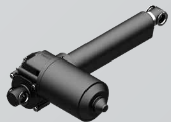
RE5004 Quiet high power actuator. Housing in composite. Max. push force: 6000N Max. pull force: 4000N Build-in length: 144 mm + stroke IP-class: IPX1
