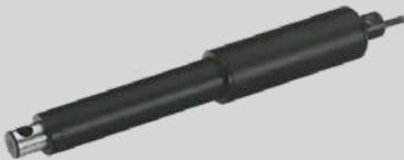
RE1000 The RE1000 is a strong inline actuator. Build in length will vary depending on the variant. Max. push/pull force: 2000N Build-in length: 155–176 mm + stroke IP-class: IPX4
